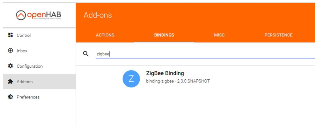
Once installed you can go to the **Configuration->Things** section of the menu and add new *Thing*. Select **ZigBee Binding -> Ember EM35x Coordinator** and then Configure it properly:
